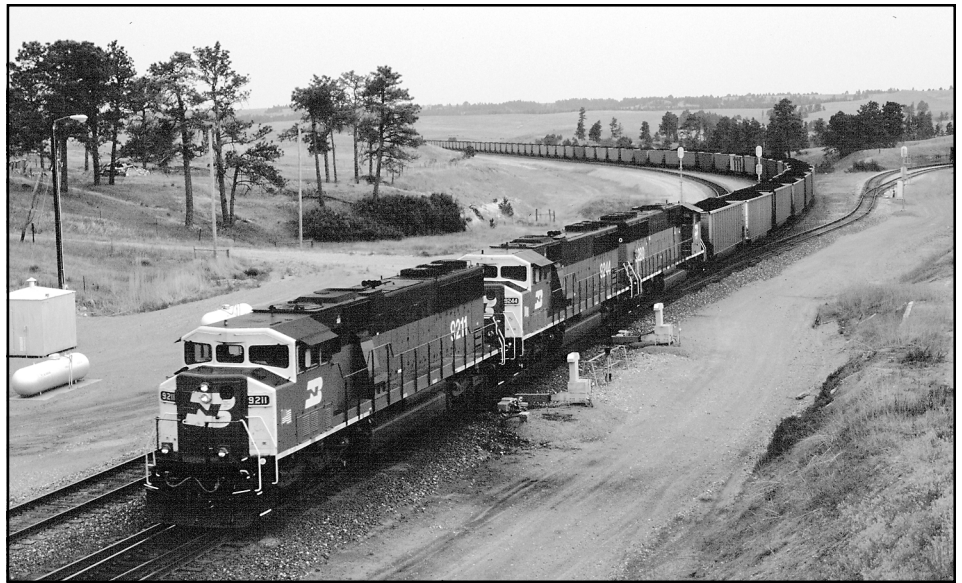
Helper locomotives 9280, 9244 and 9211 cut off on the fly at the summit of Crawford Hill at Belmont, Nebraska, after helping an east bound coal train up the 13-mile climb. – Photo © Dave Goss.
